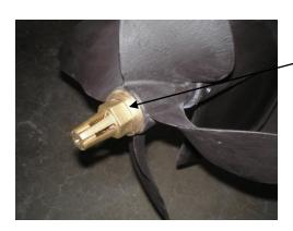
The propeller is held onto the shaft using a bronze nut and a carter pin. Remove the carter pin and then the nut. Hold onto the prop with one hand and loosed with a wrench with the other hand as shown.
