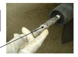
The last and very important part of the propeller assembly is the electrolysis Zinc protector attached to the bronze nut with one crew.
