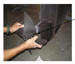
The prop will not need a special tool for removal. Pull prop off by hand or if necessary tap gently the blades close to the hub with a rubber mallet to loosen.
