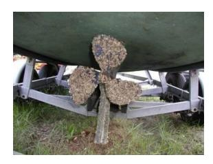
Barnacles on the prop causes vibrations and slows down top speed up to 40%.
