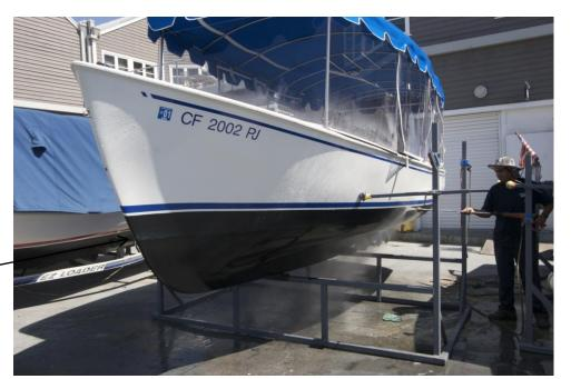
Pressure washing or hand scrubbing the bottom is a must before re-coating with paint. Immediately clean off barnacles and algae after hauling out of the water. Do not let the bottom dry out. Cleaning becomes ten times more difficult after the algae and barnacles dry out.
