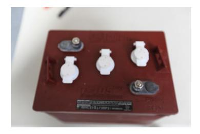
There are three cells in a six volt battery each one is a maximum finished charge voltage of 2.5 for a total of 7.5 volts. The supply voltage (under load) at full charge will be 2.14 volts per cell.
