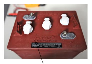
The Trojan six volt T-105 battery will put out 75 amps for 115 minutes. This battery would be considered a 225 amp rated.
