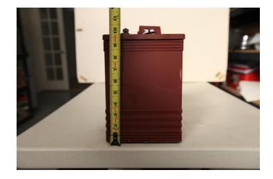
Deep cycle batteries have a reservoir of space near the bottom that makes them taller than starting batteries. The plates inside are thicker than auto batteries too. Deep cycle batteries will charge back up from being discharged without harming permanently. The small amount of oxide that sloughs off the plate lands in the reservoir space and does not come into contact with the plates, keeping them from shorting out. Since the plates are thick they can survive many cycles before they fail.
