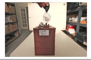
1250 to 1275 indicates a full charge. As the battery ages 1250 will be the highest level which is normal. 1225 is half, 1100 is empty. Expect over 900 cycles if battery is not discharged more than 50%. Below 50% expect 350 cycles or less.
